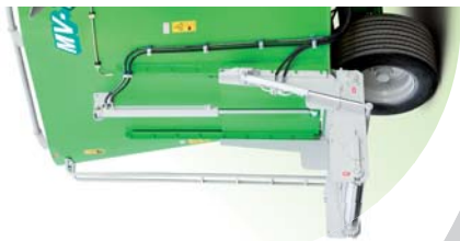
elevator on side door
