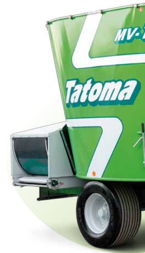
detail back conveyor
