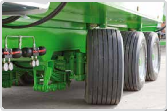
Tridem steering forced (standard equipemnt on MV 40 and 45)
