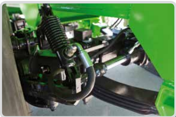
Tandem steering axle on MV30 and 35 (optional forced steering)
