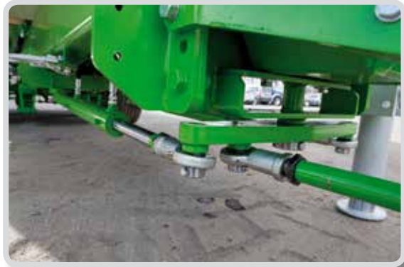
Tridem steering forced (standard equipemnt on MV 40 and 45)
