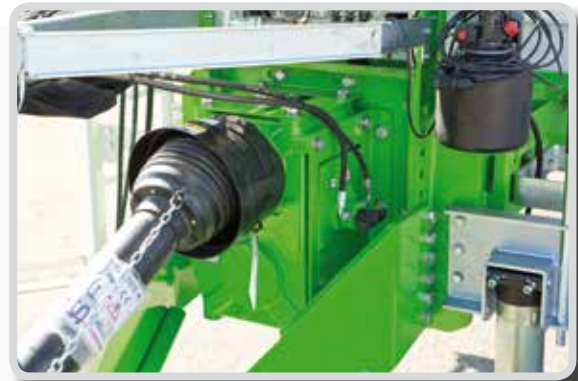
Electric hydraulic 2 speed gear box
