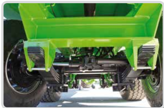
Tandem steering axle on MV30 and 35 (optional forced steering)
