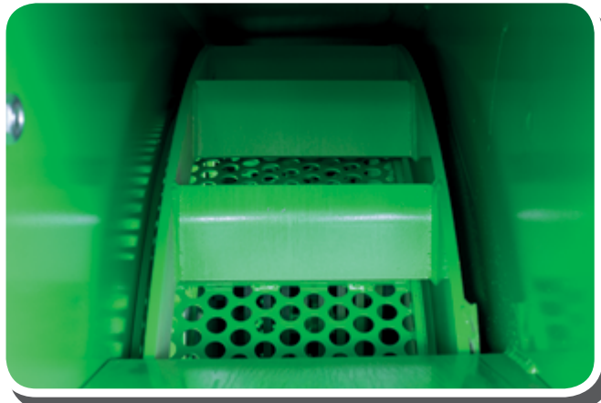
Detail mesh Ø 2,5-3 cm. And chopping hammers (inner view)
