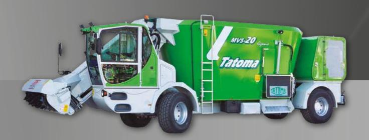
Front-axle levelling is performed by a hydraulic suspension. The rear-axle is connected by a chassis with leaf spring and rocker suspension. The first axle is for steering and driving, the second for driving and steering, allowing the machine exceptional manoeuvrability despite its size. The maximum turning angle is 40 °. The service brake is located on the first and second axle and measurements of all wheels are 445/65
