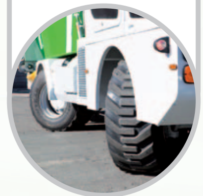
TRACTION Front axle drive and steering. Optional dual wheel drive and dual axle steering.
